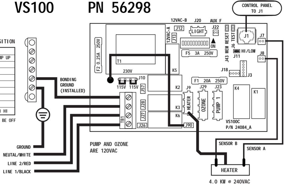
FOR HARDWIRED INSTALLATIONS, A DISCONNECTING MEANS MUST BE INSTALLED WITHIN SIGHT FROM THE EQUIPMENT AND AT LEAST 5 FEET (1.52 M) FROM THE INSIDE WALLS OF THE POOL, SPA, OR HOT TUB.
