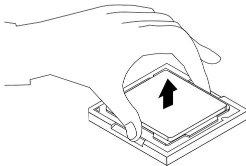
Figure 43. Removing the microprocessor
