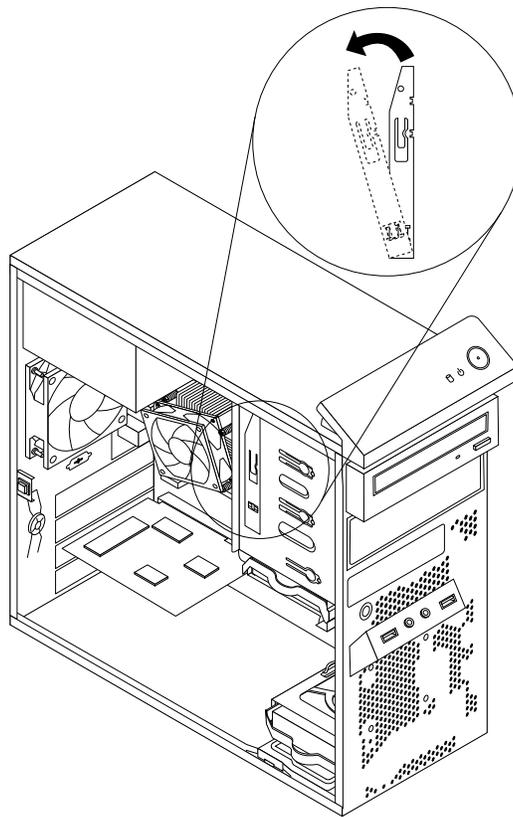
Figure 31. Removing the card reader retainer
