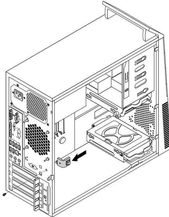
Figure 74. Installing the new cover presence switch
