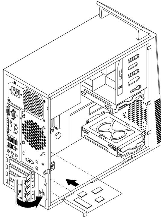
Figure 16. Installing a PCI card
