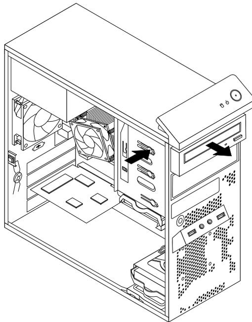
Figure 20. Removing the optical drive
