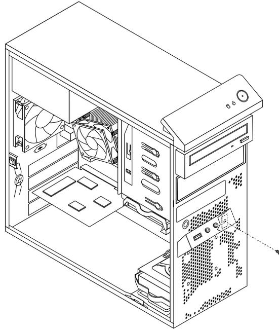
*Figure 66. Removing the front audio and USB assembly*
