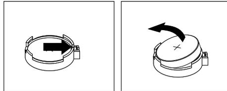
Figure 38. Removing the old battery
