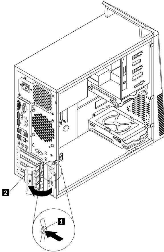
Figure 14. Opening the PCI card latch
