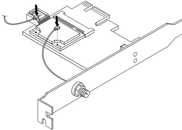
Figure 83. Installing the Wi-Fi antenna cables
