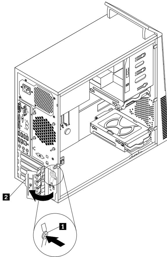
Figure 76. Opening the PCI card latch
