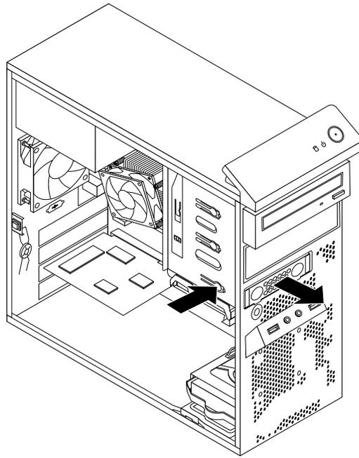
*Figure 48. Removing the mSATA solid-state drive storage converter*
