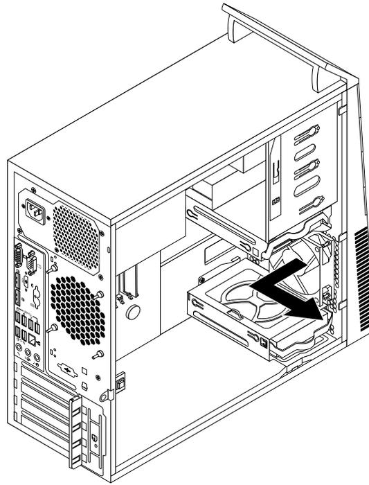
*Figure 62. Removing the front fan assembly*
