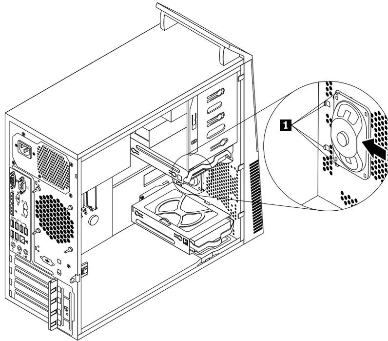
Figure 70. Installing a new internal speaker
