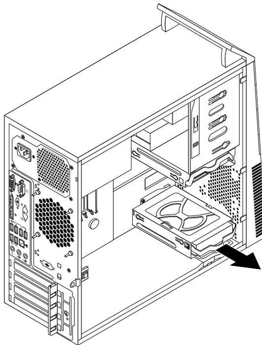
Figure 57. Removing the secondary hard disk drive
