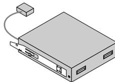
Figure 32. Installing the card reader retainer
