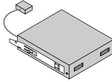
Figure 36. Installing the card reader retainer
