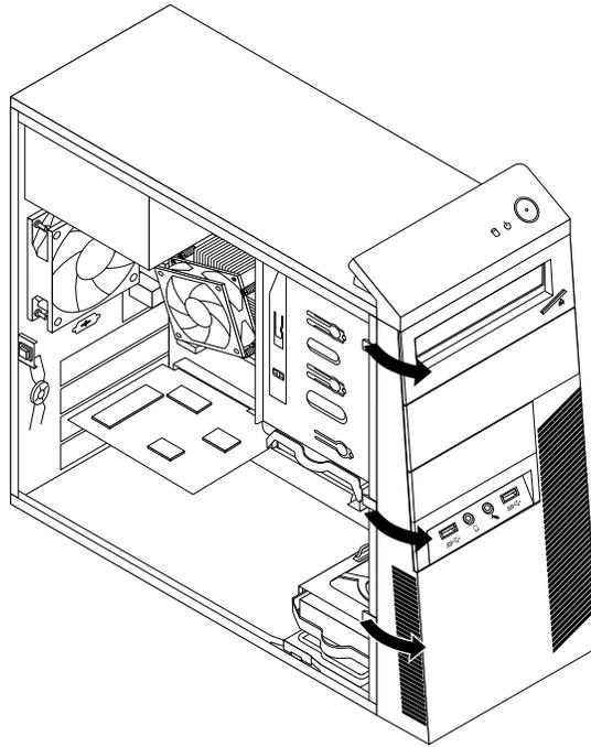
Figure 13. Removing the front bezel
