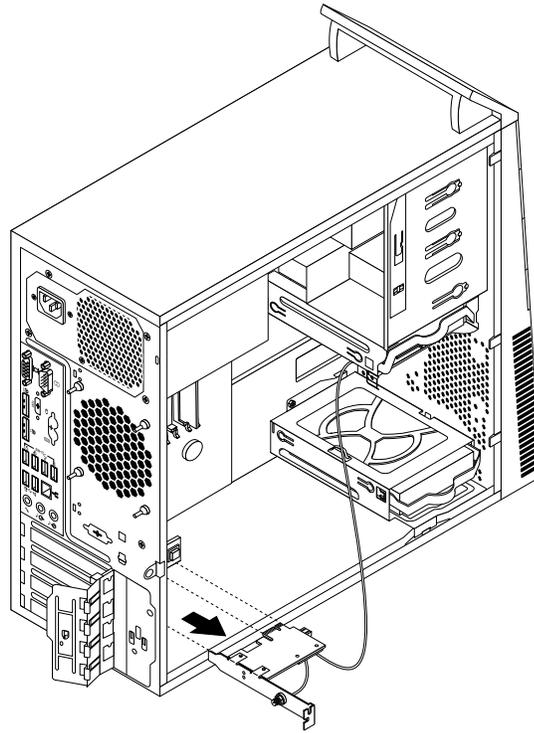
Figure 77. Removing the Wi-Fi adapter card
