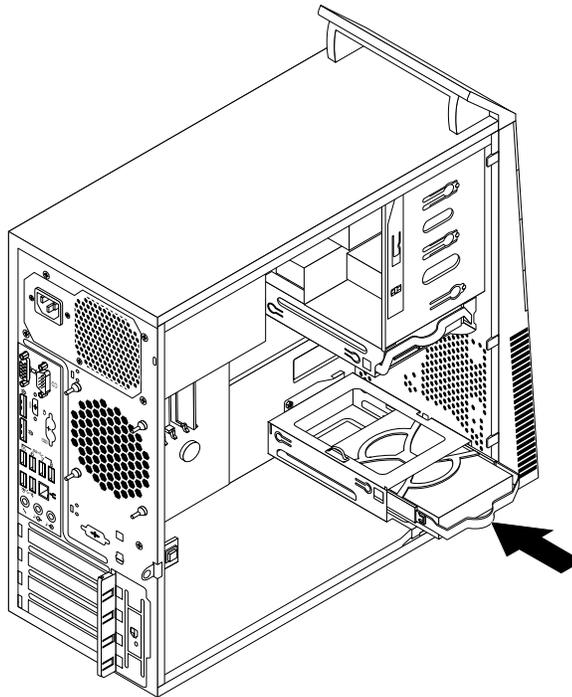
Figure 59. Installing the secondary hard disk drive
