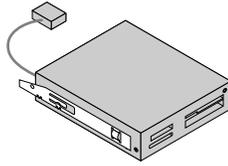
Figure 29. Installing the card reader retainer
