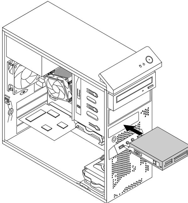
Figure 30. Installing the card reader
