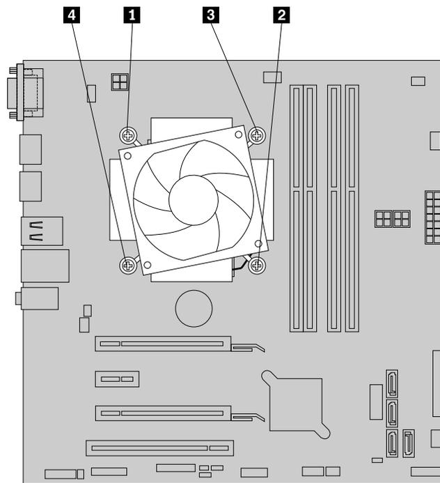
Figure 41. Removing the heat sink and fan assembly
