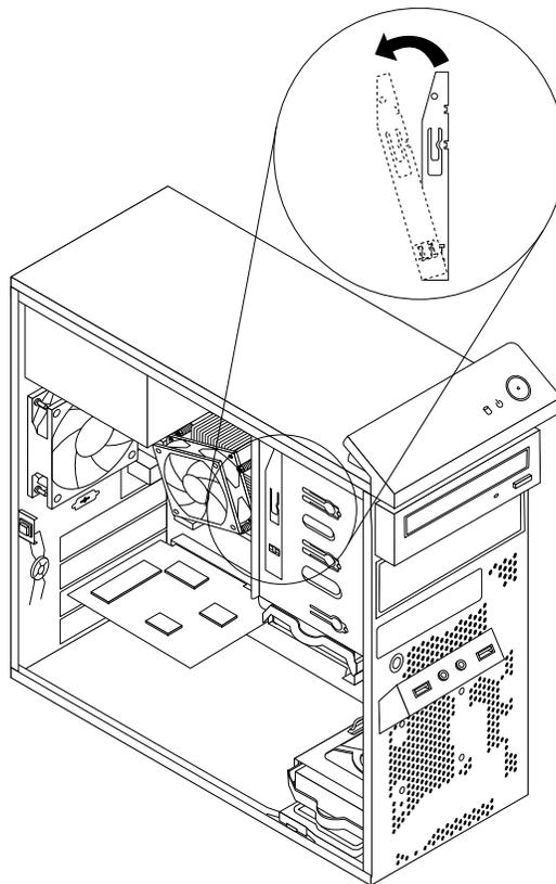
Figure 24. Removing the card reader retainer
