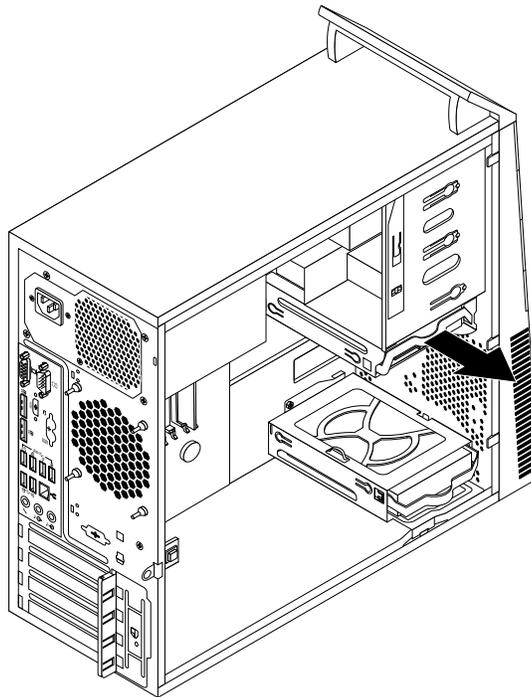
*Figure 54. Removing the primary hard disk drive*
