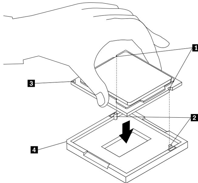
Figure 44. Installing the microprocessor
