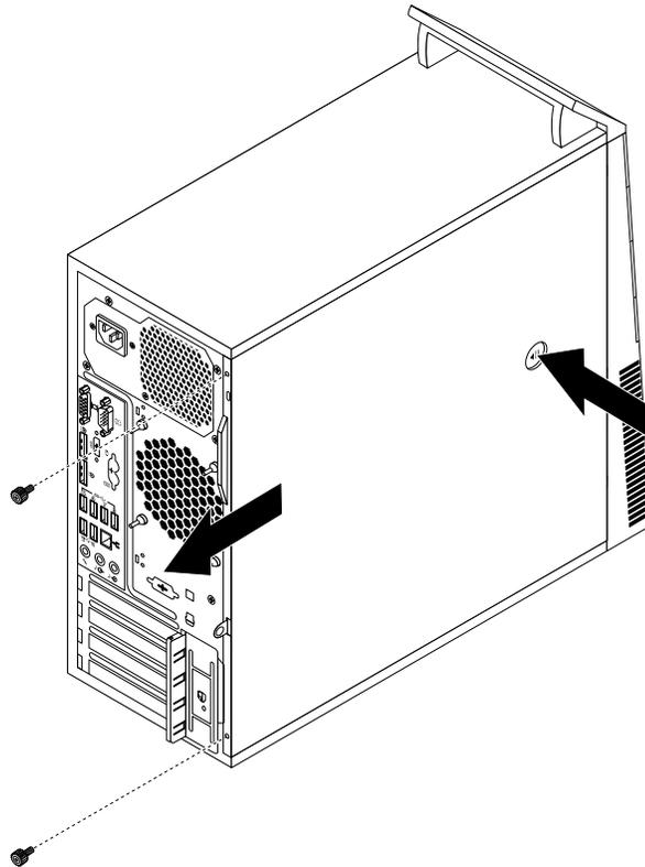
Figure 12. Removing the computer cover
