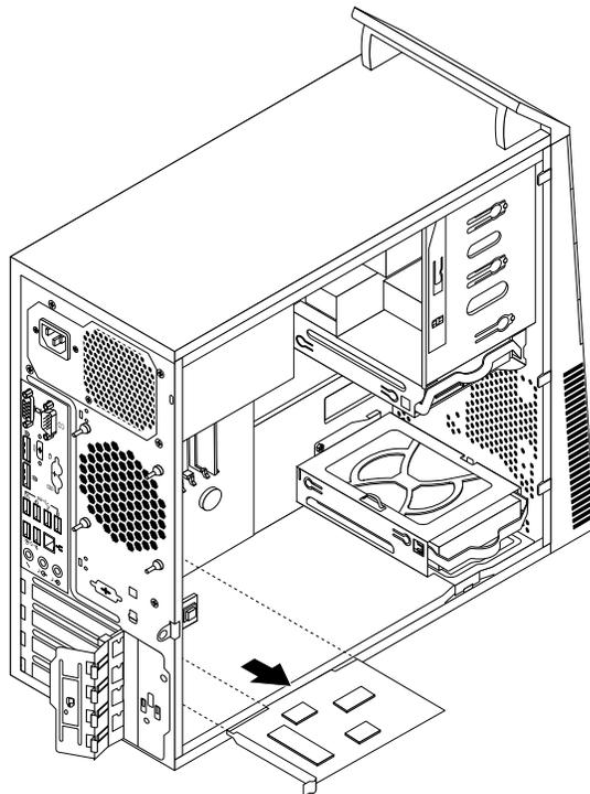
Figure 15. Removing a PCI card
