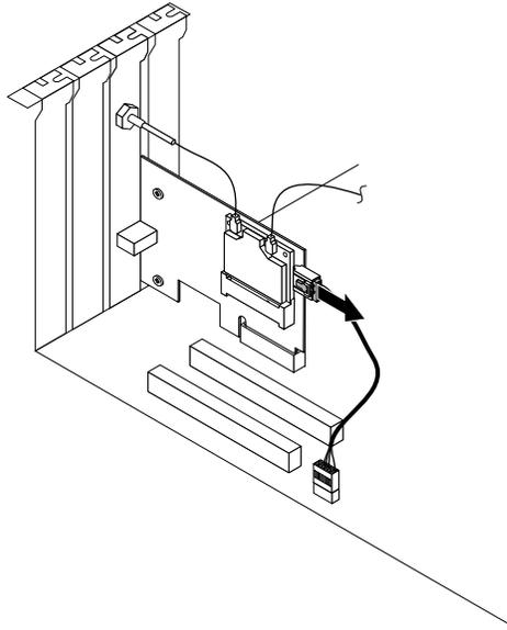
*Figure 75. Disconnecting the Bluetooth cable*
