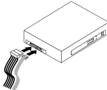
Figure 23. Connecting the optical drive
