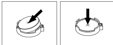
Figure 39. Installing a new battery
