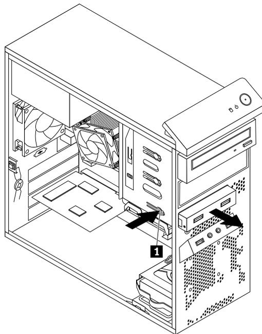
Figure 35. Removing the front USB assembly
