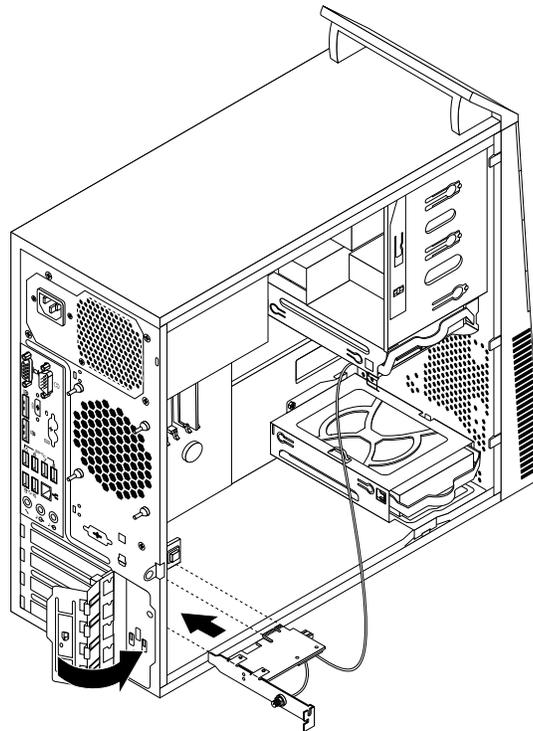
Figure 84. Installing the Wi-Fi adapter card
