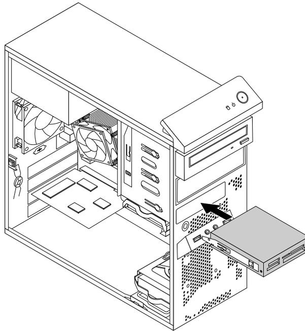
Figure 26. Installing the card reader
