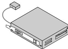
Figure 25. Installing the card reader retainer
