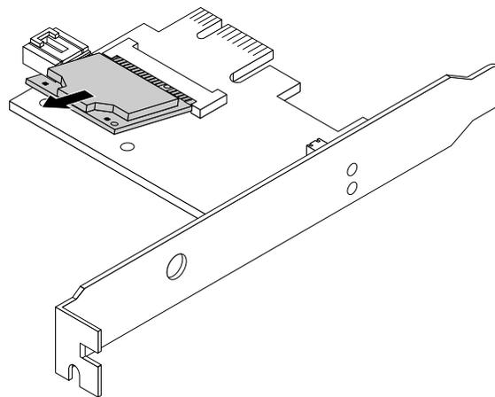
*Figure 80. Removing the Wi-Fi card module*
