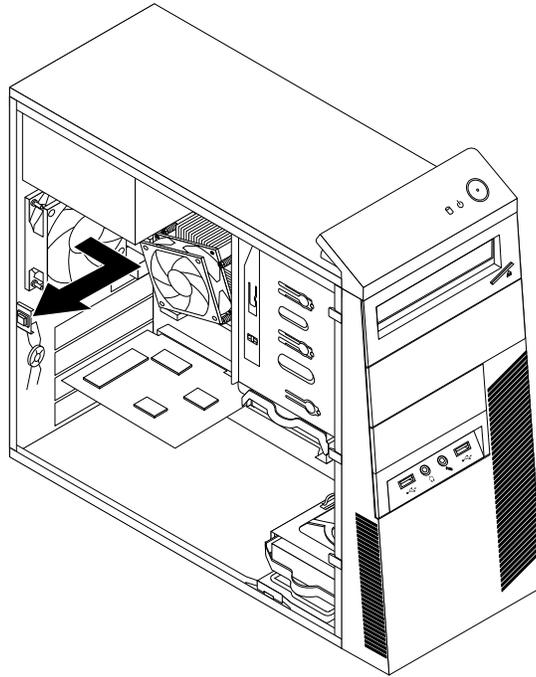
*Figure 64. Removing the rear fan assembly*
