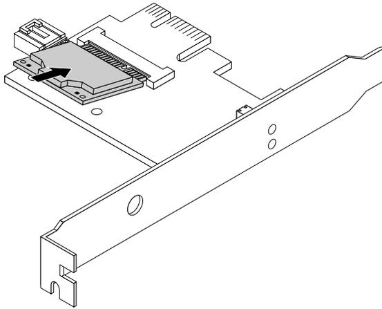
Figure 81. Installing the Wi-Fi card module
