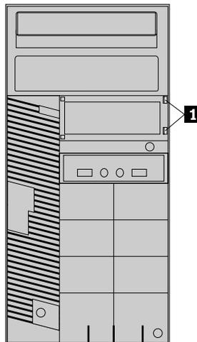
Figure 34. Removing the card reader cover
