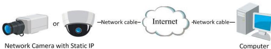
**Figure 2-5** Accessing the Camera with Static IP Directly
