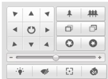
Figure 5-2 PTZ Control Panel
