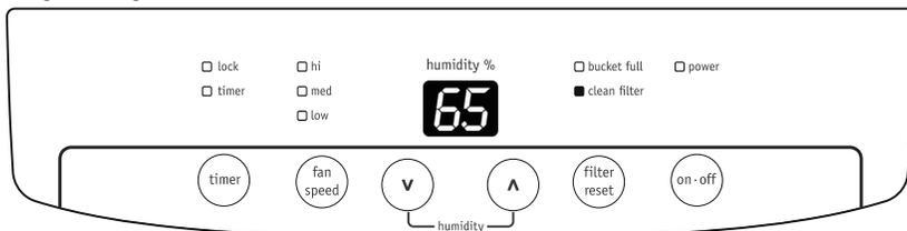
6. The TIMER function enables you to either Delay Start or Delay Stop the unit in the choice from 0.5 hour to 24 hours. If the unit is running, then selecting Timer will turn the unit off in the hours that will be set (Delay Stop). If the unit is off, then selecting Timer will turn the unit on in the hours that will be set (Delay Start).
