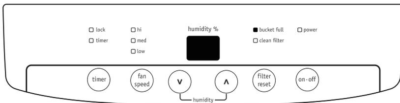
2. To turn the unit on, press the ON/OFF button. The unit will run in the factory setting of CONTINUOUS and high fan speed. In the CONTINUOUS mode, the unit will only display CO and not the room humidity. It is recommended you leave the unit running in the CONTINUOUS setting for the first three or four days until the sweating and dampness odors have stopped.
