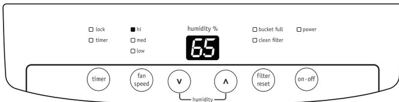
5. The CLEAN FILTER light will illuminate after 250 hours of operation. At this time refer to the care and cleaning section to remove and clean the filter. Once the filter has been cleaned and replaced, simply press the FILTER button to extinguish the light.
