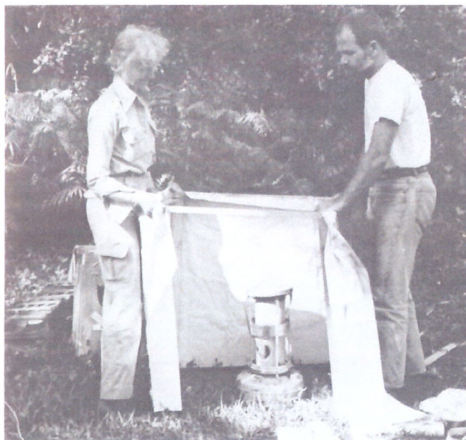
Canvas skirt around the aluminum drying frame keeps heat from escaping except through stack of specimens. Note Aladdin stove beneath.
